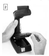
Fig. 12: Removing the battery compartment
