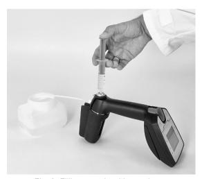
Fig. 8: Filling sample with a syringe
