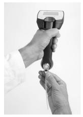
Fig. 2: Connecting the filling tube
