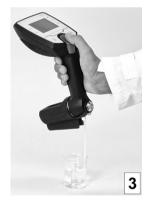
Fig. 7: Filling sample with the filling tube
